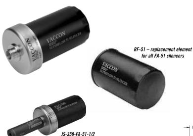
The FA-51 Series silencers offer remarkable noise reduction for high volume exhaust applications without causing back pressure. These silencers are ideal for quieting large air valves that must exhaust quickly to maintain high cycle rates. Vaccon uses the FA-51 silencers on all high flow venturi vacuum pumps where even a small amount of back pressure would decrease performance.
