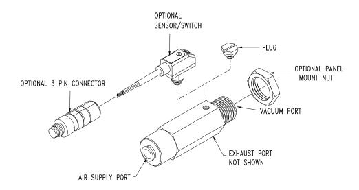
Vaccon's VPI-90H in-line venturi vacuum pump features the air supply port and vacuum port on the same axis. Unlike standard venturi vacuum pumps where the vacuum port is 90° from the supply port, the VPI-90H's can be attached vertically to a robotic end of arm tool in a single or densely populated array to accommodate any size, shape and weight of product being handled.
