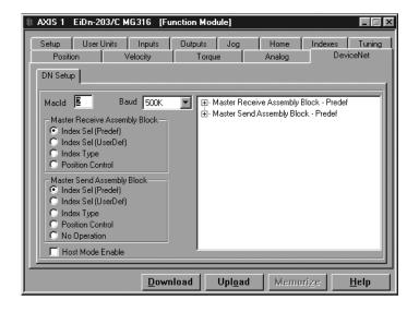
Change the nature of the pre-configured assembly blocks by simply changing the mapping of the DN bits. The DN Bits are user defined bits that can have different I/O functions mapped to them.
