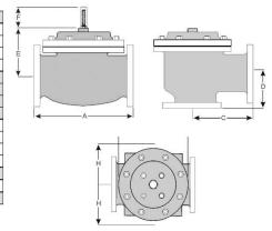
For maximum efficiency, the Apollo control valve should be mounted in a piping system so that the valve bonnet (cover) is in the top position. Other positions are acceptable but may not allow the valve to function to its fullest and safest potential. In particular, please consult the factory before installing 8" and larger valves, or any valves with a limit switch, in positions other than described. Space should be taken into consideration when mounting valves and their pilot systems.
